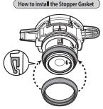
Fit the gasket into the lower groove of the inner stopper, paying attention to the top and bottom.
